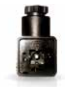
1578501 Quick connection connector DIN 43650, suitable for all IM2 coils. Cable gland Pg9 (cable diameter 6 \div 8 mm). Pg11 cable gland thread; Adjustable cable outlet in 4 positions every 90^\circ .
